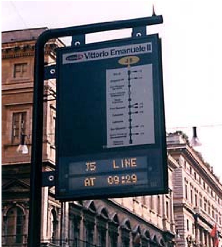
Figure 1. Real-time Arrival Sign with Static and Dynamic Elements
